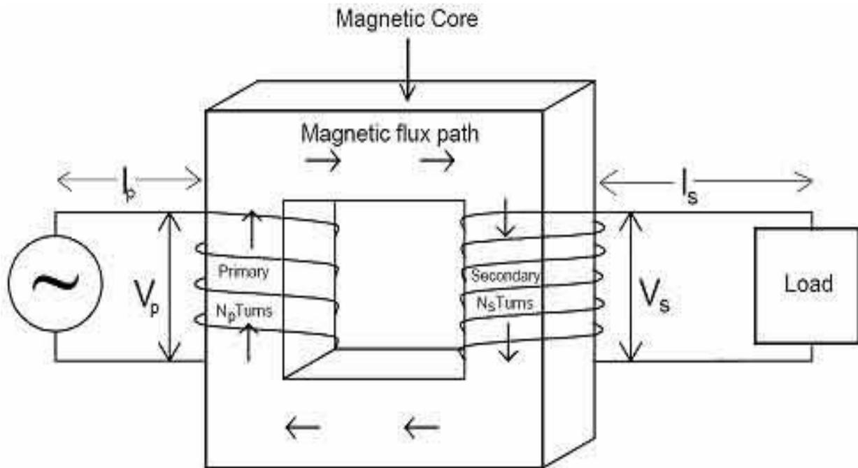
An alternating voltage ( $V_p$ ) applied to the PRIMARY creates an alternating current ( $I_p$ ) through the primary.
