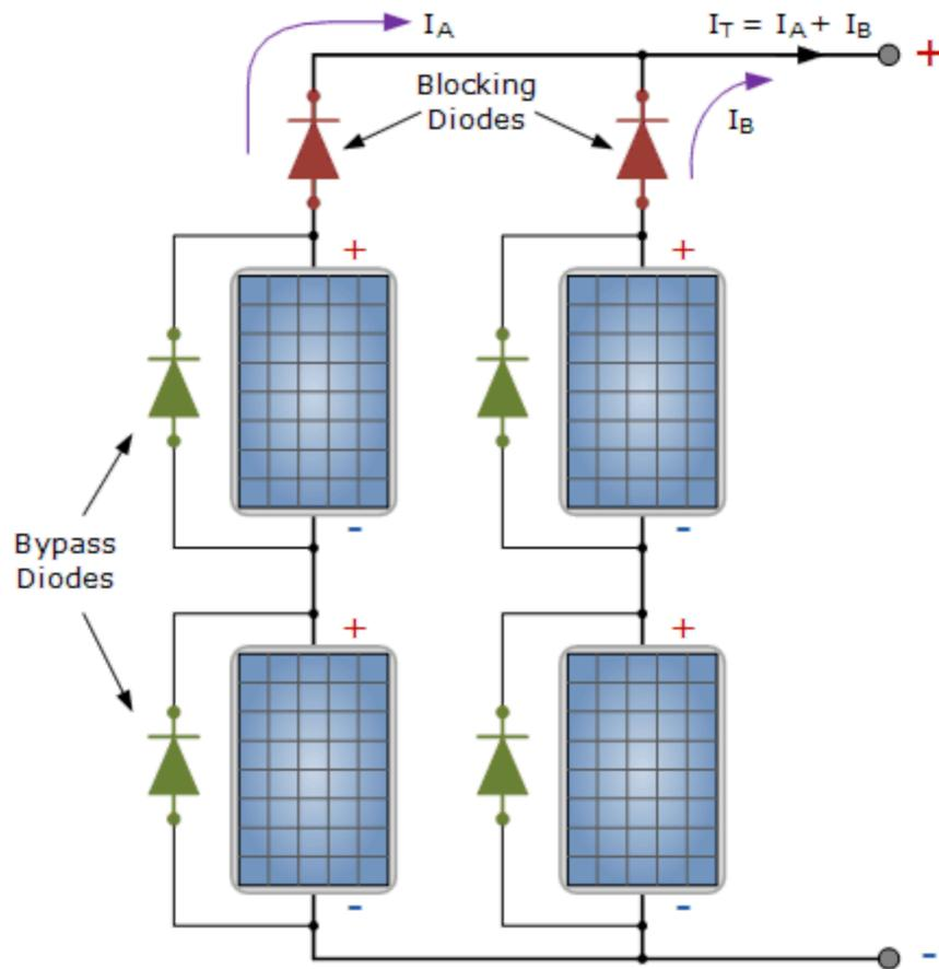
As we said earlier, *diodes* are devices that allow current to flow in one direction only. The diodes coloured green above are “bypass diodes”, one in parallel with each solar panel to provide a low
