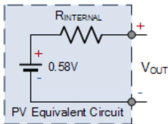
The equivalent circuit of a PV, shown on the left, is that of a battery with a series internal resistance,  $R_{INTERNAL}$ , similar to any other conventional battery.
